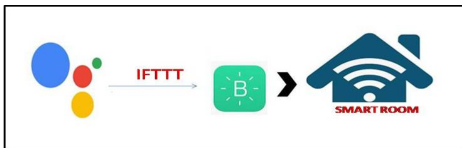
Fig. 2. Use of Google assistant to develop smart room with the help of BLYNK
